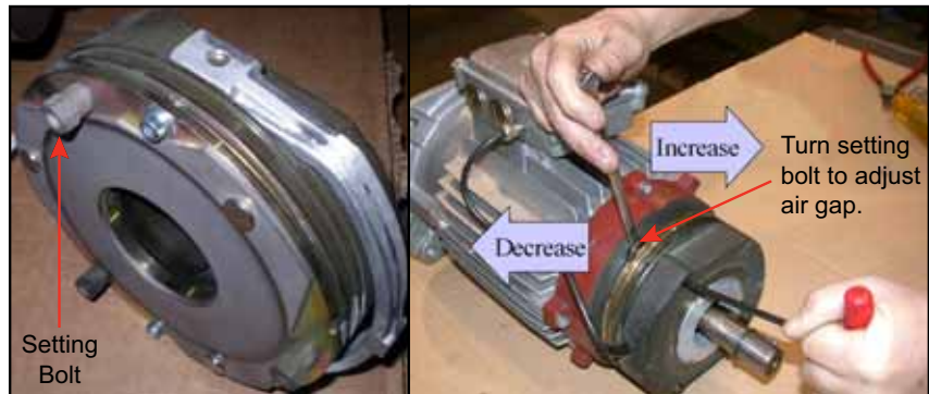
Figure 6-25: Adjusting the Setting Bolt
